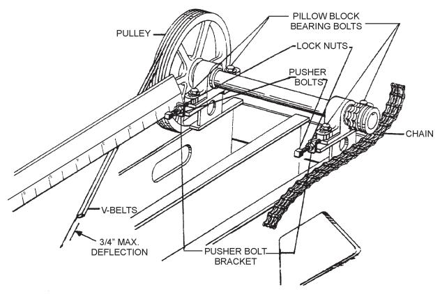
Figure 27. V-Belt and Drive Chain Adjustment
